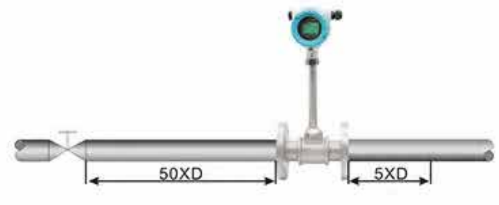
Regulating Valve, Half-open Gate Valve
